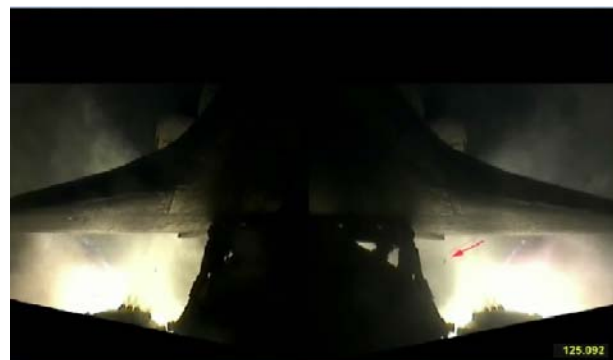
Figure 6. STS-116 In-Flight Anomaly of TPS Striking the Orbiter during SRB Separation.
