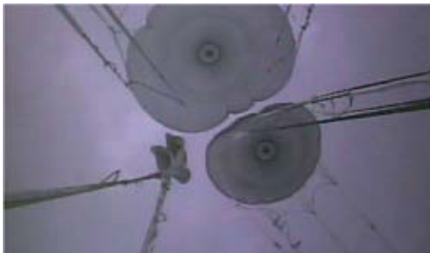
Figure 5. STS-122 Parachute Failure Observed With Parachute Forward Skirt Dome Camera.
