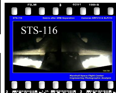
BTA from Aft BSM Hits Orbiter
