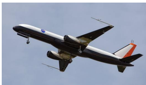
Figure 7. T-2 subscale jet transport aircraft Credit: NASA Langley Research Center
