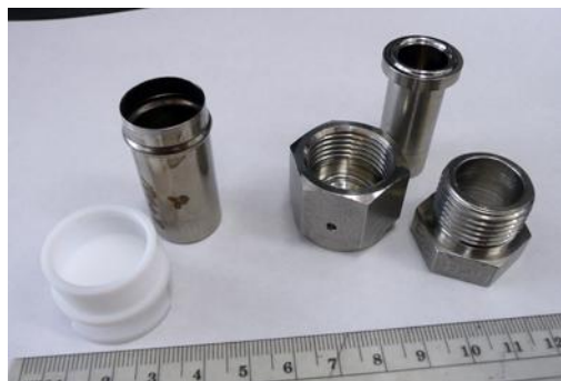
Fig. 1 On left is a drawn stainless container with Teflon snap cap currently used in JSC curation for rock and regolith (lunar and meteorite). On right is UCB low organic container fabricated from stainless steel vacuum flange (3 pieces). Scale is in cm.
