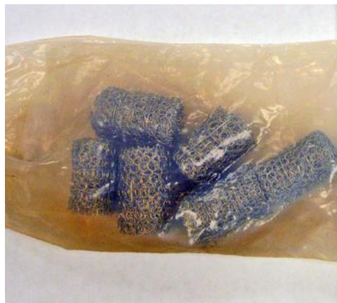
Fig. 3. Woven aluminum mesh used as organic monitor during Apollo. Mesh rolls are about 1-inch across, contained in a Teflon film bag..
