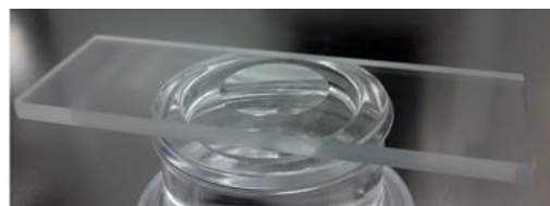
Fig. 2. Small Stardust and Hayabusa grains are cleanly contained when placed in a dimpled glass slide sandwich.
