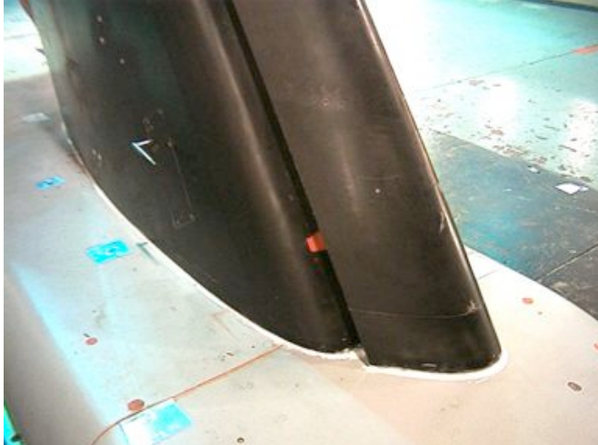
Figure 13. Forward probe at \eta = 15\% as mounted in the 14x22.
