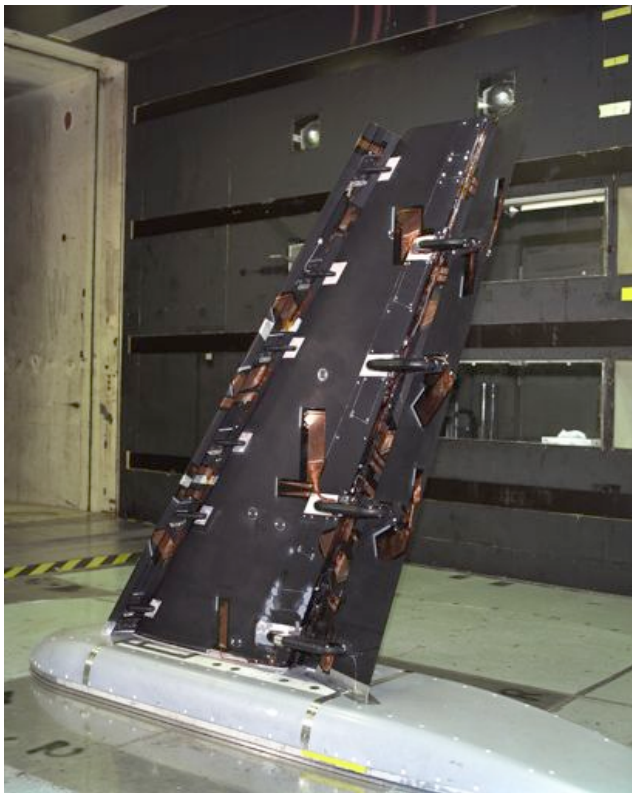
Figure 3. Trap Wing model installed in 14x22 during 2002 test.
