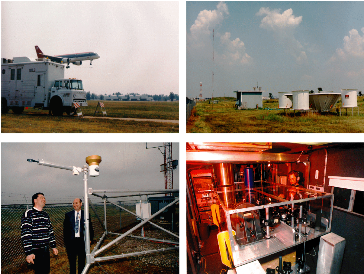
Figure 3. Memphis Wake Vortex Field Experiment. A B757 landing in the background of the NASA lidar van (top left); profiler (top right); Michael Mathews (left) and Dr. Fred Proctor (right) standing next to the radiometer mounted at the base of the meteorological tower (bottom left); and Dr. Tim Dasey in the lidar van (bottom right).
