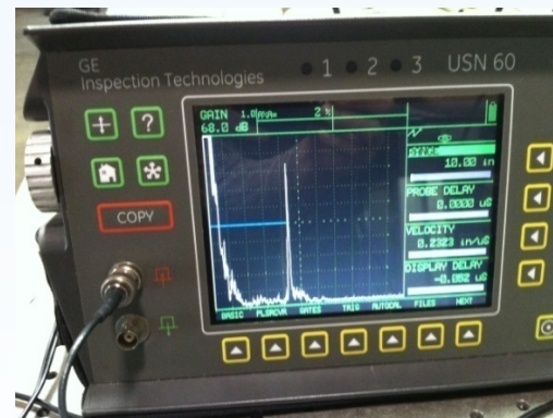
Surface wave ultrasonic NDI technique
