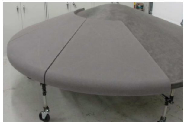
Figure 8. Fit check of TPS modules on 2.65-m aeroshell.
