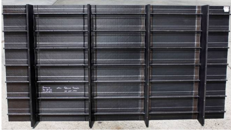
Figure 3.—Example PRSEUS panels.
