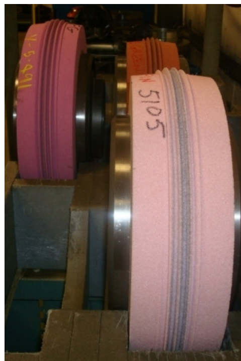
Figure 7.—Grinding wheels configured for face gear grinding.
