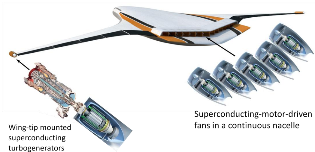
Figure 1 N3-X Hybrid Wing Body(HWB) Aircraft with a Turboelectric Distributed Propulsion (TeDP)
