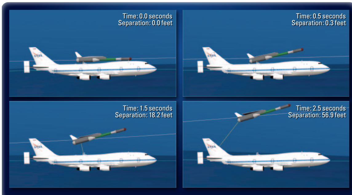
Separation simulation snapshots for a Flight Test Demonstrator
