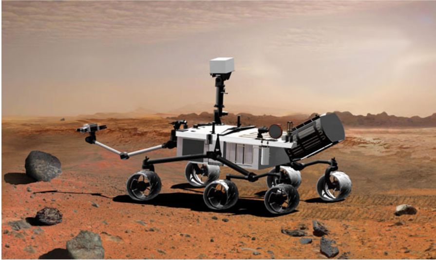
Fig. 11. Artist's concept of the Mars Science Laboratory (MSL) Curiosity rover with the MMRTG shown attached to the back end (right side in the picture). MSL is ~3 m long (not including the arm), 2.7 m wide, 2.1 m tall with a mass of 900 kg. The arm can reach about 2.1 m. (Image credit: NASA/JPL/Caltech).
