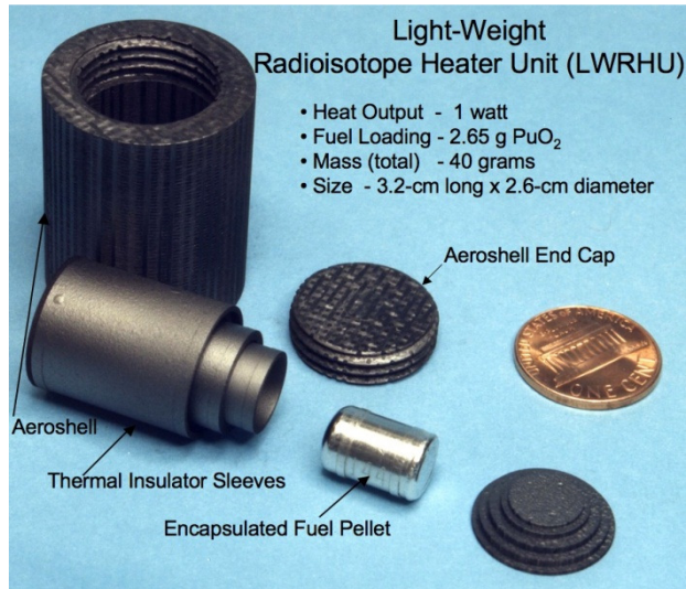
Fig. 4. Light-Weight Radioisotope Heater Unit (LWRU) (DOE)
