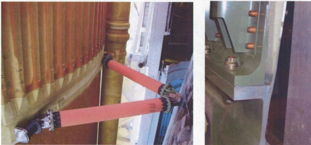
Figure 1. A view of Space Shuttle External Tank LH 2 intertank flange area on Orbiter attachment side is shown on the left. A cutaway of the intertank flange area showing the crevice is given on the right.
