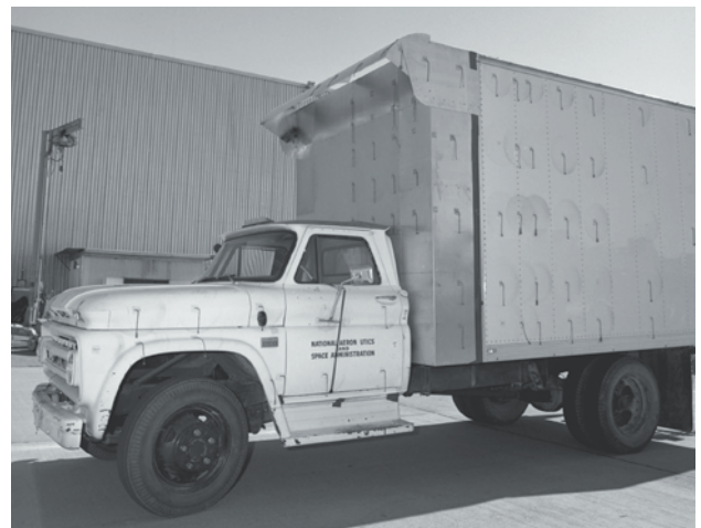
Center engineers tested the two-axle truck with a device called a "flow vane" attached to the front of the cargo box roof. They tried three configurations of the flow vane. Tufting is a good indicator of the device's benefit. NASA
