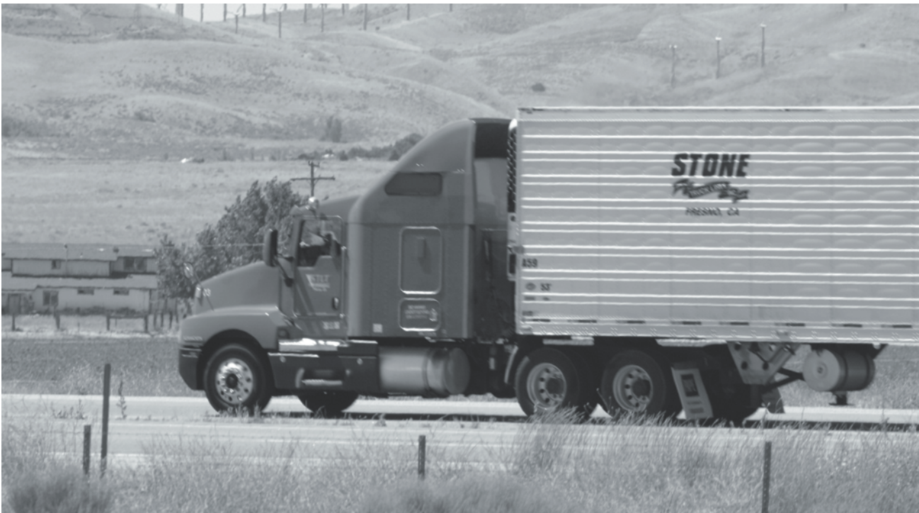
This picture of a Kenworth T600, the first production tractor with aerodynamic fairings of real consequence, reveals a fairing arrangement echoing that of the Bat Truck.
