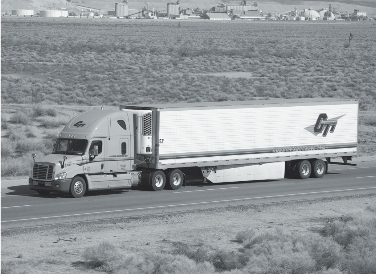
A late model Gordon Trucking, Inc. tractor-trailer unit featuring a well-faired cab and trailer side skirts.
