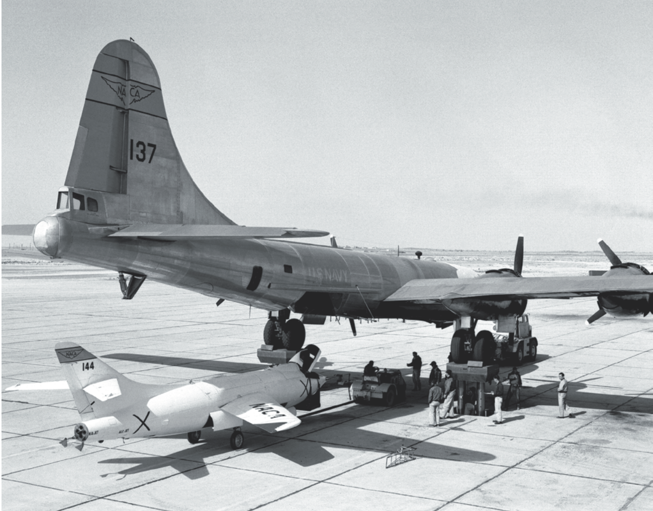
The Douglas D-558-2 being loaded into the belly of the mothership. Like the X-1, it was rocket-powered, and it was the first aircraft to exceed Mach 2.
