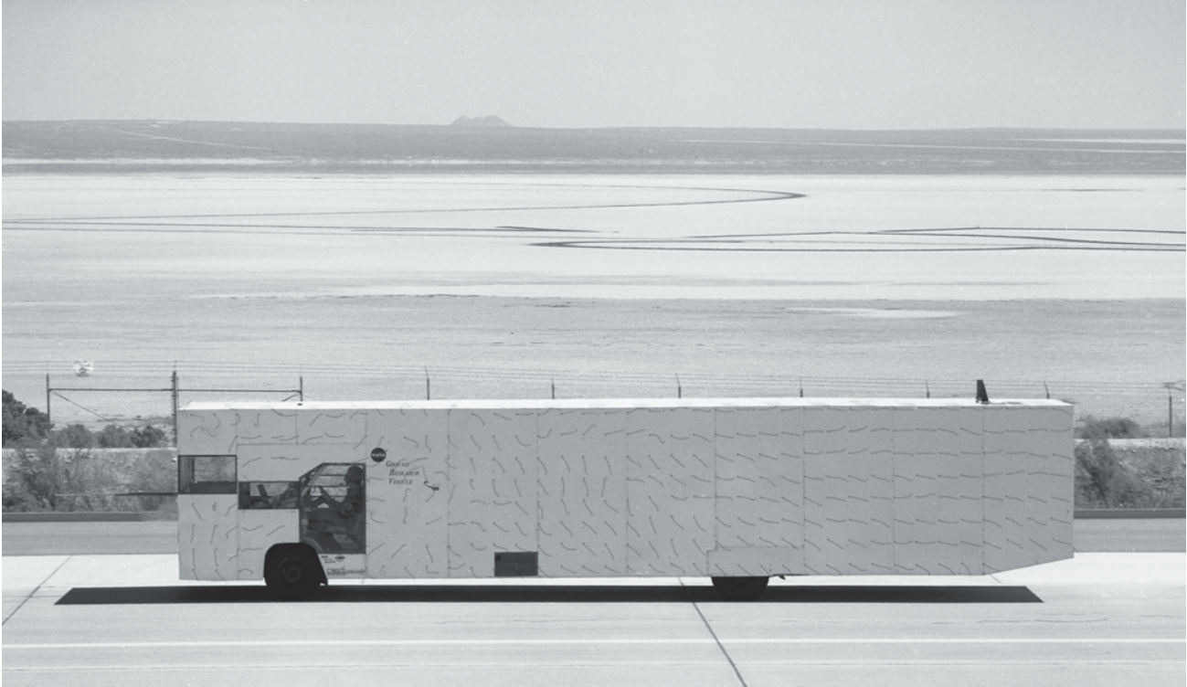
Above and below, the Ground Research Vehicle (Roadrunner) during runs on the NASA Dryden flight line. Tufts of yarn show chaotic airflow over the vehicle's first half but fairly smooth and controlled airflow over the latter half. A rake, used to measure boundary layers, stands above the roofline at the vehicle's aft end.
