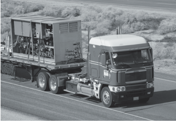
At left, a cab-over-engine tractor, a style increasingly rare on American highways for aerodynamic reasons but one that retains advantages in certain environments. The image at right is of a conventional tractor.
