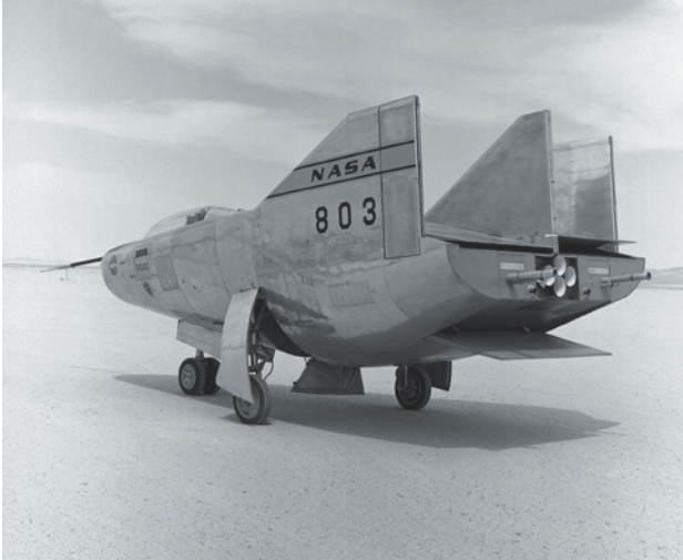
The back end of the Northrop M2-F3, highlighting the blunt aft end and the rocket nozzles.
