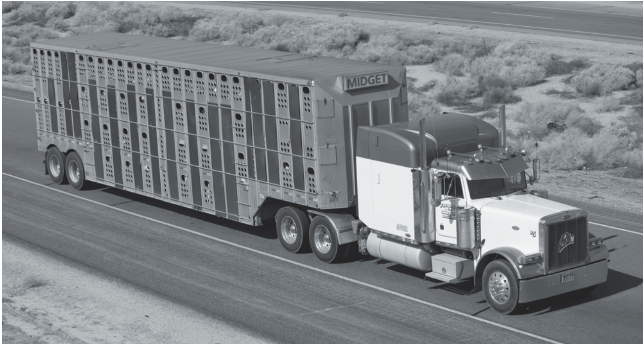
A conventional tractor-trailor pulling a typical livestock hauler. The tractor makes little to no concession to aerodynamics.
