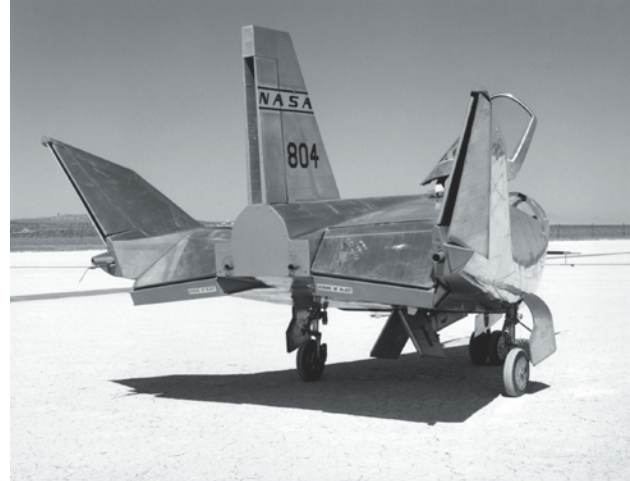
The Northrop HL-10, seen from the rear, before the rocket motor had been installed (beneath the center vertical stabilizer). This angle illustrates the blunt base so typical of lifting bodies, but does not reveal the amount of increased drag produced when control surfaces are deployed on descent (re-entry). In that event, inboard and outboard surfaces of all three vertical surfaces deploy, as do the top and bottom “flaps” on the body, dramatically increasing drag.
