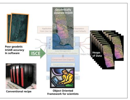
The InSAR Scientific Computing Environment (ISCE) replaces old InSAR processing algorithms and conventional computing paradigms with modern geodetically accurate algorithms embedded at the core of a modern, flexible, and extensible object-oriented computing framework. The framework enables scientists to easily and efficiently process raw data into useful data products for their science models and investigations.
