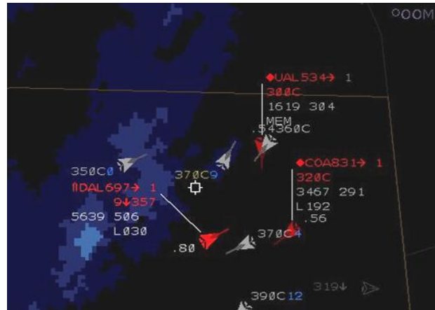
Figure 13. short-term conflict caused by an unexpected early descent of one aircraft and vectoring solution
