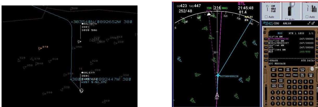
Figure 9. A trial-plan prepared by the controller (left), then sent to the flight deck as an FMS-loadable message (right)
