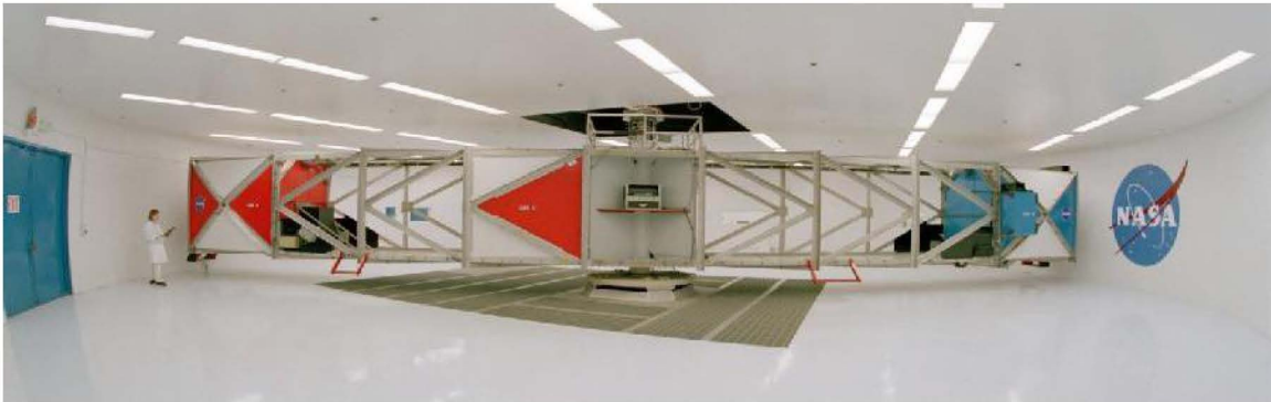
NASA Ames Human Centrifuge Configured with Cab A (left) and Cab B (right)
