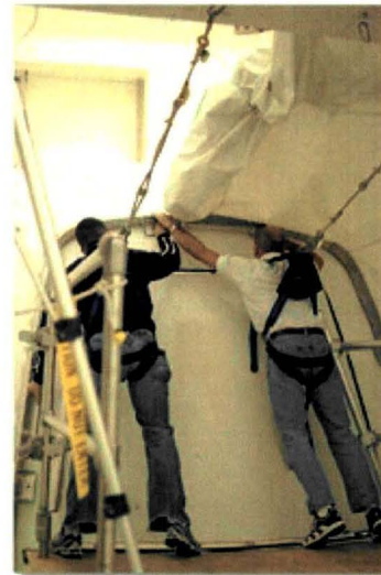
Figure 10 – "White Room" to Ogive Fairing Interface
