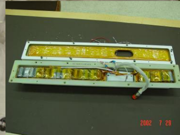
Simplified Aid For EVA Rescue (SAFER) Battery Lithium Manganese Dioxide (Li-MnO 2 )
