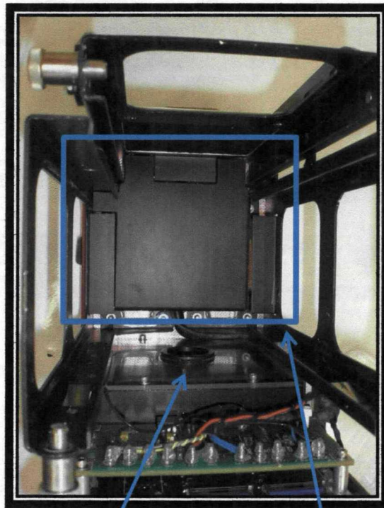
Airflow Duct (in proper position)
