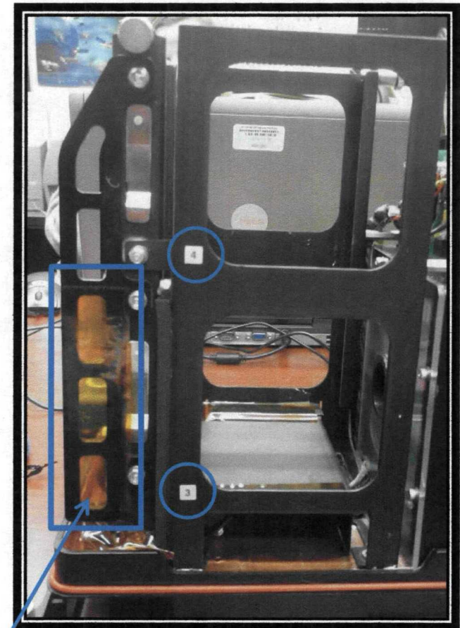
Kapton Tape covering outside slotted frame on the 3, 4 side
