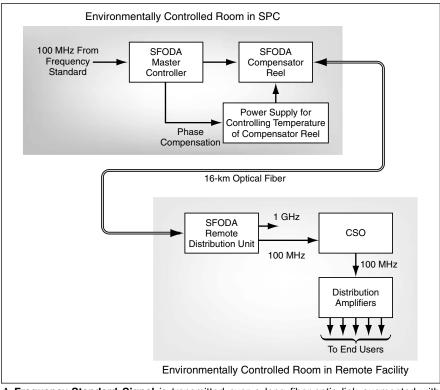
A **Frequency-Standard Signal** is transmitted over a long fiber-optic link augmented with equipment at both ends that stabilizes the output frequency and phase to a high degree.
