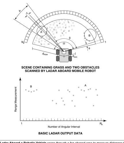
Ladar Aboard a Robotic Vehicle scans through a fan-shaped area to measure distances to nearby objects, which are represented here by circles. The small circles represent stalks of grass. Large circle A represents a tree trunk partly hidden by grass; large circle B represents a tree trunk in the clear.
