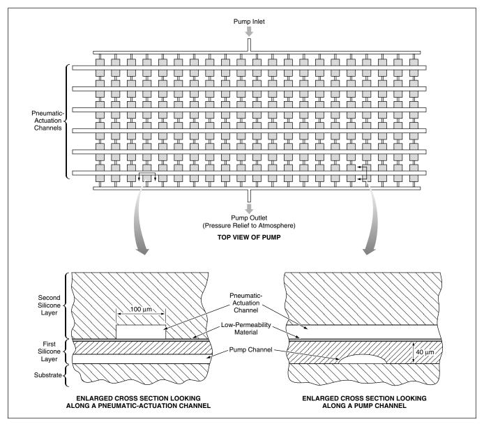
**Pneumatic-Actuation Channels** would be alternately pressurized and depressurized to push down the silicone arches or allow them to spring back up, respectively. This action would create waves of opening and closing, equivalent to peristalsis, that would move gases along the pump channels. The dimensions shown here are exemplary, not exclusive.
