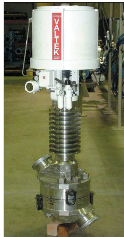
The Split-Body Design of this valve accommodates changes in trim. The heat-exchanger fins help keep the plug stem packing warm enough to function at cryogenic temperatures.
