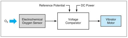
The **Comparator Triggers the Motor** into operation when the partial pressure of oxygen, measured by the sensor, falls below a preset value represented by the reference potential.
