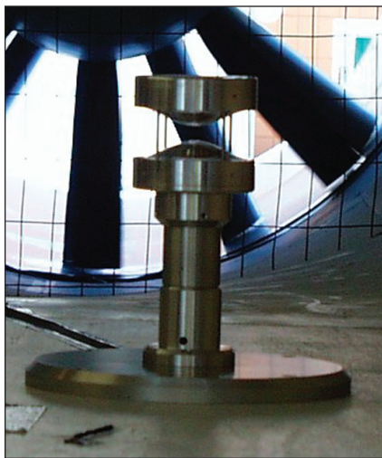
Figure 1. A Prototype Three-Dimensional Venturi Sensor is shown here mounted in a wind tunnel for testing at Embry-Riddle Aeronautical University, FL.
