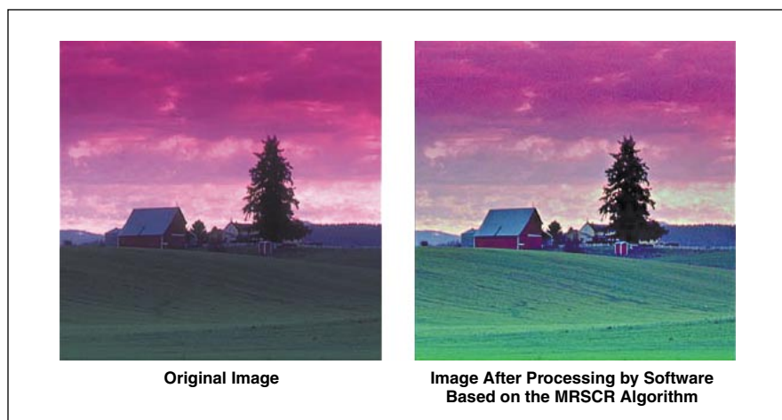
Details in Shadows are more readily perceptible after processing by software based on the MSRCR algorithm.
