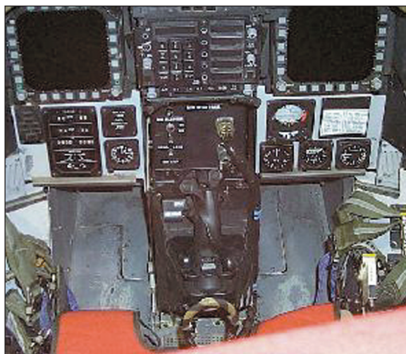
The Ministick is shown here installed in the aft cockpit of the F/A-18 airplane.
