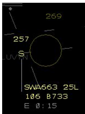
Figure 2. Aircraft with target location outside slot marker.
