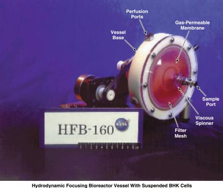
Figure 1. The Hvdrodynamic Focusing Bioreactor utilizes rotation and viscosity to generate hydrodynamic forces for controlling locations of cells and bubbles while maintaining low shear.
