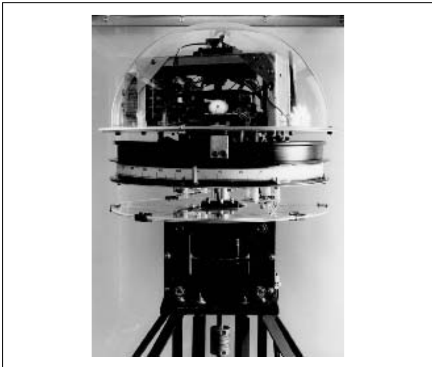
Figure 1. Transformers, Instead of Slip Rings and Brush Contacts, are used to couple ac power and data signals between stationary and rotating circuits.
