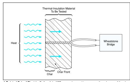
A Twisted Pair of Electrically Insulated Wires can be used to measure the advance of the char front in real time: The intermittent short-circuit resistance of the twisted pair, as measured by the Wheatstone bridge, varies with position of the char front.
