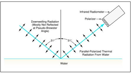
An **Infrared Radiometer** would be aimed toward water at the pseudo-Brewster angle and would respond to radiation polarized parallel (but not perpendicular) to the plane of incidence.
