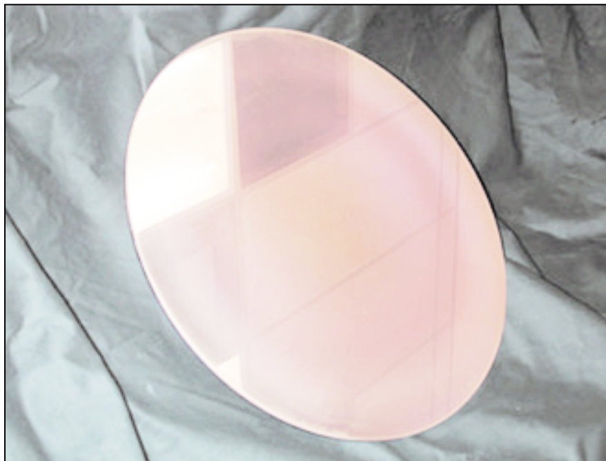
A Cu/Cu 2 Zr, Nanolaminate was fabricated on a super-polished low-thermal-expansion glass form.
