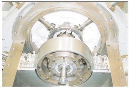
The **High-Temperature Switched-Reluctance Electric Motor**, capable of operating at a speed of 8,000 rpm at a temperature of 1,000 °F ( $\approx$ 540 °C), is a modified version of a magnetic bearing capable of operating at 15,000 rpm at 1,000 °F ( $\approx$ 540 °C).
