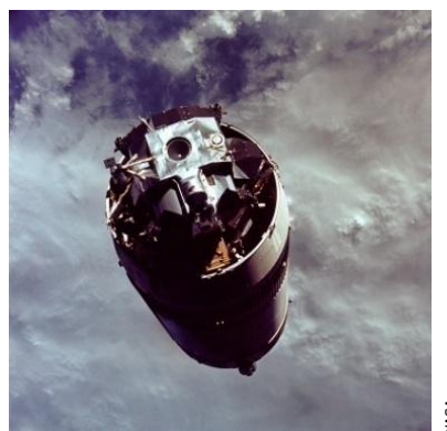
Figure 4.4 Apollo 9 view of LM and S-IVB during the transposition maneuver (March 1969).
