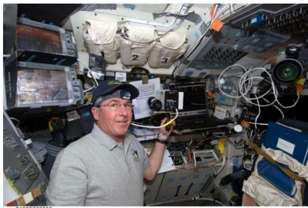
Figure 25.13 Mission Specialist Steve Robinson photographed on the port side of the aft flight deck. The primary RPOP laptop is to the right of him and he holds an HHL unit. Above left of Robinson is a CCTV screen with a ranging ruler overlay. Above that is another CCTV screen for the centerline camera, also equipped with an overlay. Robinson used the LED headlamp to read procedures in the low-light environment on the flight deck. Photo taken before MC-3 and around the time the first HHL mark was taken.
