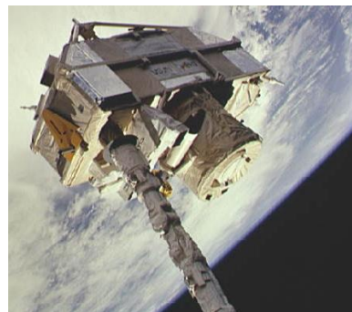
Figure 18.17 CRISTA-SPAS after being grappled by the RMS (STS-66, Nov. 1994).
