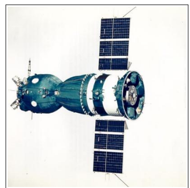
Figure 10.5 Soyuz with solar arrays during the Apollo/Soyuz mission (July 1975).
