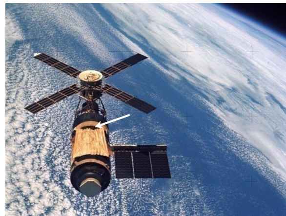
Figure 10.4 Skylab with thermal parasol indicated (Feb. 1974).
