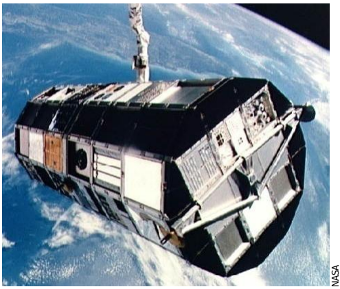
Figure 10.8 LDEF being maneuvered with the RMS.
