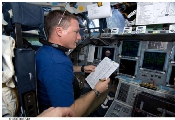
Figure 25.16 Pilot Terry Virts at the commander's station between MC-4 and +R Bar arrival. He is holding the APPROACH cue card. The RNDZ TIGs flight note and the RCS FAILURE/RESPONSE cue card are clamped to the overhead panel in front of him for easy reference. At the lower right of the photo is a laptop running a centerline camera repeater.
