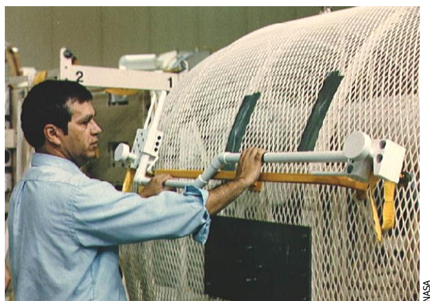
Figure 17.2 Grapple bar on a SYNCOM IV-3 mock-up in preparation for the STS-51I mission (1985).
