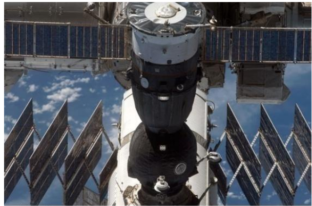
Figure 25.35 Soyuz TMA-16 photographed during the fly-around, close to the -V Bar, to check for loose MLI.
