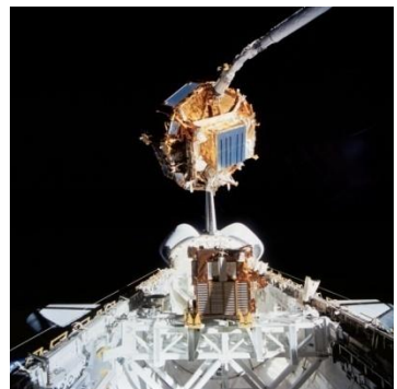
Figure 19.4 SFU about to be berthed in the payload bay of Endeavour . OAST-Flyer is below SFU (STS-72, Jan. 1996)
