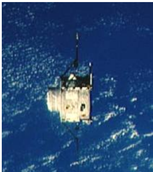
Figure 18.2 PDP after release from the RMS (STS-51F, July/Aug. 1985).
