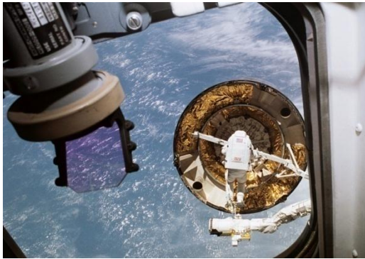
Figure 17.5 EVA crewman on the RMS attempts to capture INTELSAT (right). The COAS is on the left (STS-49, May 1992).
