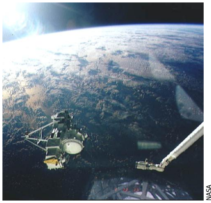
Figure 18.12 SPAS-II/IBSS after release from the RMS (STS-39, April/May 1991).
