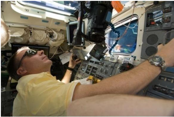
Figure 25.34 Pilot Terry Virts flying the orbiter during the later part of the fly-around, before the SEP-1 burn. Virts manipulated the Translational Hand Controller with his left hand (as shown) to control relative motion during the fly-around. His right hand is guarding the Rotational Hand Controller (not normally used) from accidental deflection by other crew members taking photos through the other overhead window. Sunglasses were worn to improve visibility of the ISS in the presence of direct sunlight while the Sun skirted the edge of the overhead window field of view.
