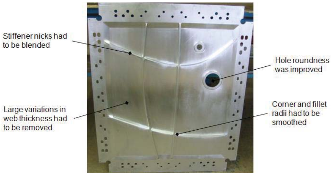
Figure 17. Picture of the Al-2139 Test Panel without Steel Tabs.
