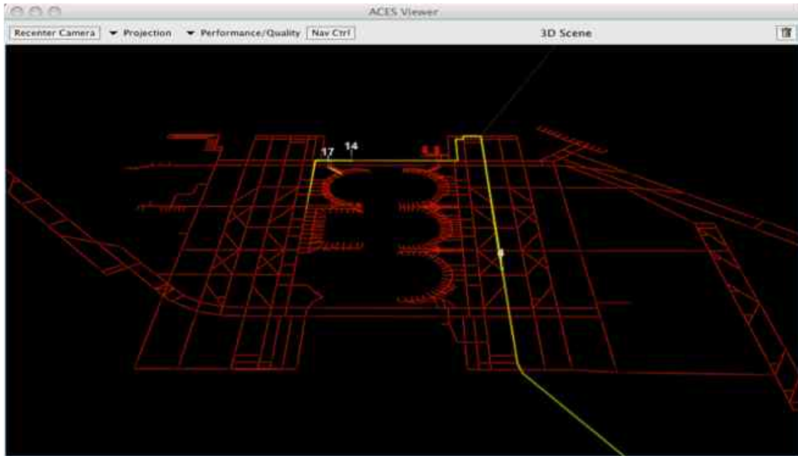
Figure 21. Dallas-Fort Worth Runways. FAA Runway data was translated into a format normally used by IV4D for visualizing a complete trajectory as a line. In this case, altitude was set at 0 feet, while latitude and longitude “waypoints” formed straight lines.
