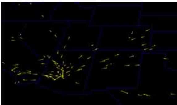
Figure 7. Default view of flight track data. Taken from a simulation of a day's worth of traffic. Only flight tracks for arrivals to and departures from Phoenix are visualized.
