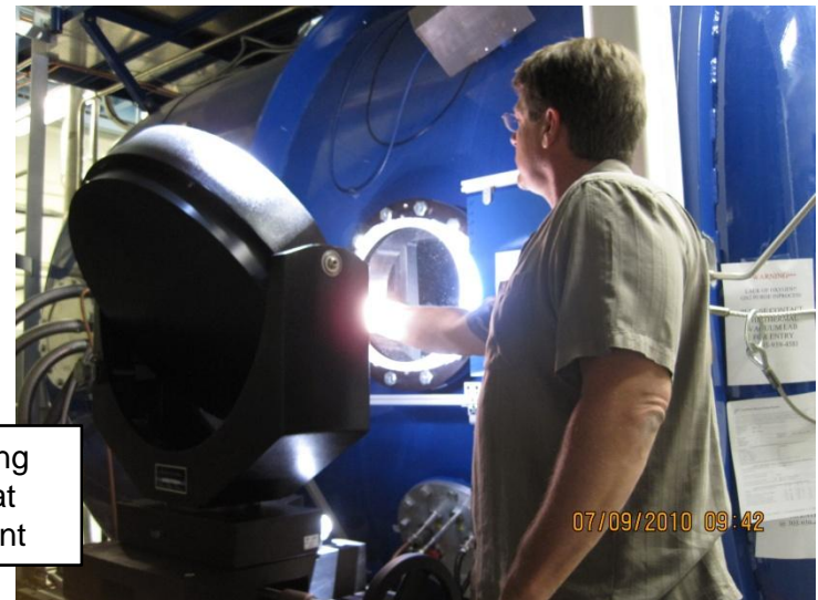
Aligning "Death Star" Calibration Sphere
