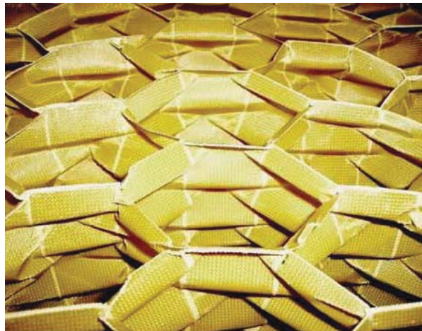
Figure 16. Close-up photograph illustrating the energy absorption modes exhibited by the DEA.
