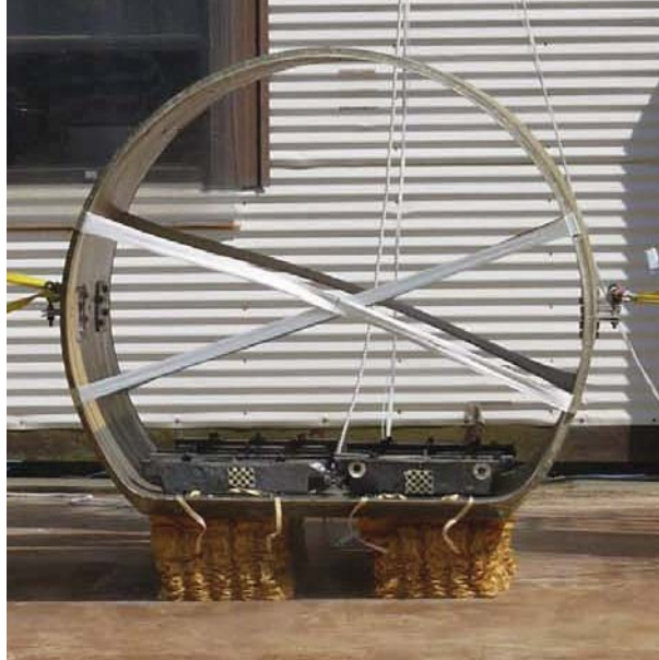
Figure 27. Post-test photograph illustrating DEA crush response.
