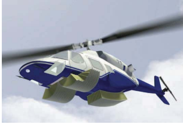
Figure 8. Artist's rendition of a rotorcraft with a set of energy absorbers deployed. The front energy absorbers are shaped to allow for egress.
