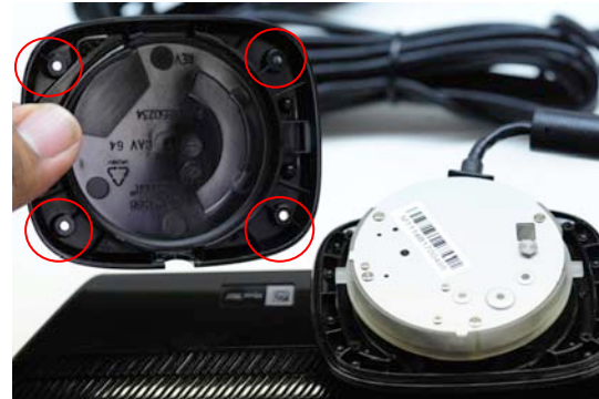
Figure 4. Removal of the Motorized base Cover. The case that houses the motor can then be removed also.
