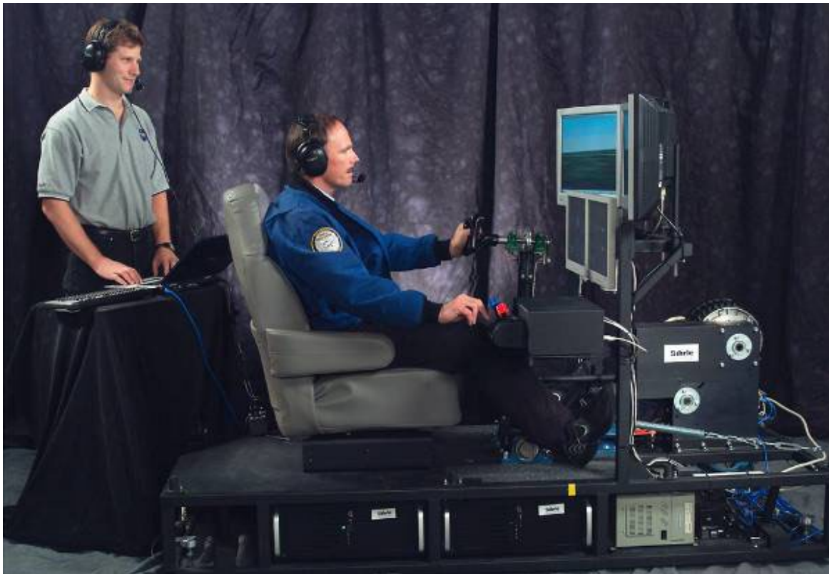
Figure 5.—NASA's Ice Contamination Effects Flight Training Device (ICEFTD).
