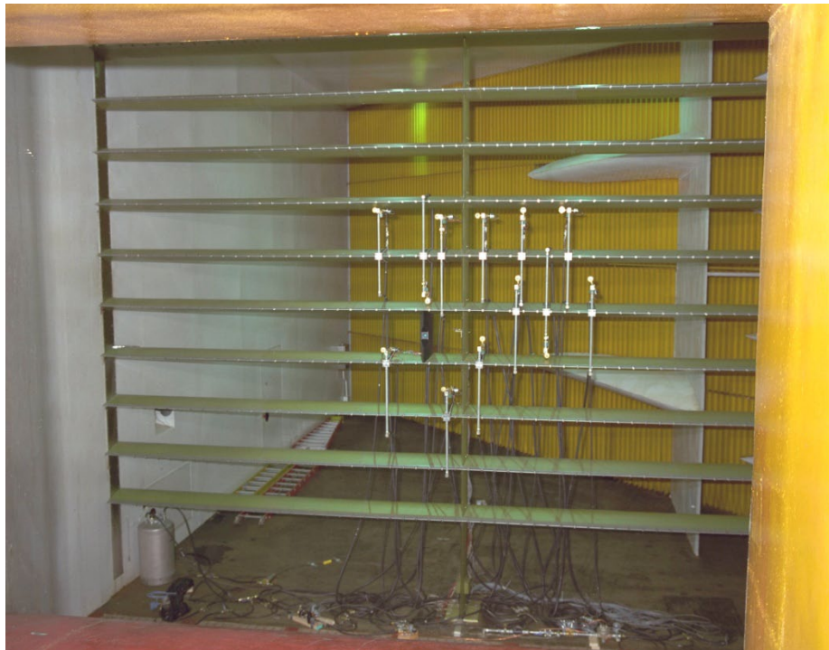
Figure 2.—Installation of spray system used for IRT impingement tests.
