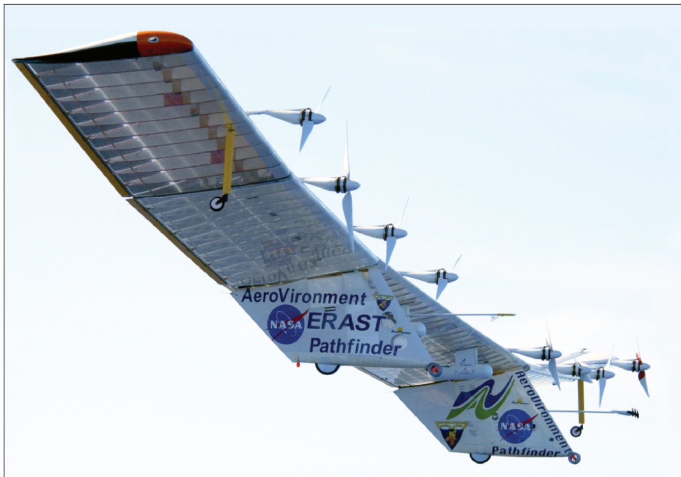
A Solar-Powered, Unpiloted Airplane includes two payload pods, on the underside of the middle section, that carry electronic cameras and telemetry subsystems.
