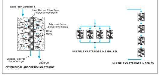
In a **Centrifugal Adsorption Cartridge**, the liquid effluent from a bioreactor is channeled along a spiral flow path through a selectively adsorbent material. The length of the spiral path contributes to efficient collection of a bioproduct suspended or dissolved in the liquid. Multiple centrifugal adsorption cartridges can be connected in series or parallel.
