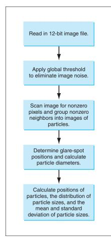
The Algorithm of the Proposed Method would process DPIV data to extract information on particle sizes. The size information would be in addition to the velocity information extracted from the data by use of previously developed DPIV software.
