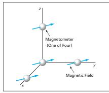
Four Magnetometers at corners of a cube provide noisy, redundant measurements of a magnetic field. The redundancy can be used to partly correct for the noise contributions.
