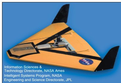
Information Sciences & Technology Directorate, NASA Ames Intelligent Systems Program, NASA Engineering and Science Directorate, JPL Photograph shows the Biomorphic Flyer Platform . The platform was successfully demonstrated in 2001.
