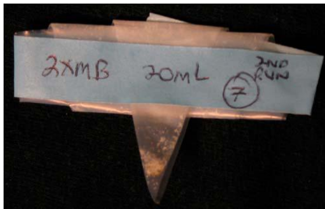
Figure 5. Salt precipitates produced in the Mars evaporites apparatus. Approximately 50 mg of evaporites were formed from 20 ml of brine. Salts were sealed in the conical Teflon sleeves by folding and taping the wide end. The sealed sleeves were then shipped to the Planetary Electrical Properties and Geophysics Laboratory at Southwest Research in Boulder, Colorado, for infrared spectral analysis, and to the Institute for Meteoritics at the University of New Mexico for SEM and microprobe analysis.
