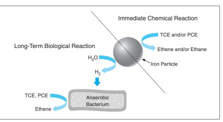
An **Injected Iron Particle** causes the reduction of chlorinated hydrocarbons (especially TCE and PCE). These compounds are converted to hydrocarbons along two reaction pathways: an immediate chemical reduction and a long-term biological reduction.
