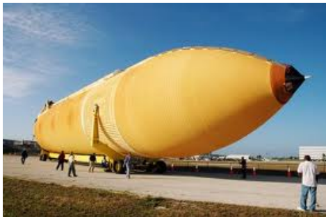
Figure 4: The External Tank rolls from the barge docked in the turn basin to the VAB. Photo credit: NASA
